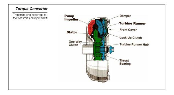
A **torque converter** is a type of fluid coupling, which allows the engine to spin somewhat independently of the transmission. Trucks with torque converter are proved to be more capable of accelerating in difficult conditions such as great slopes than the simple ones.
